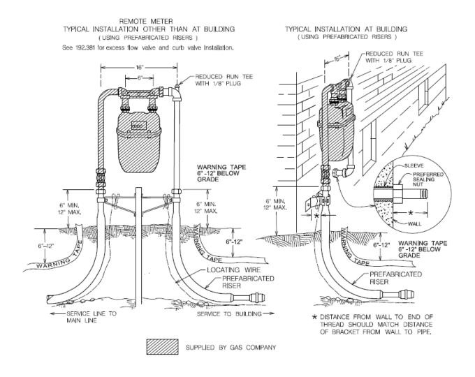
Note: Consumer to end service line 6" to 12" above finished grade. Meter to be installed by Peoples.
