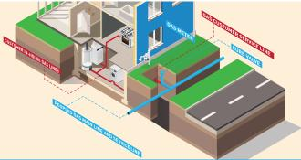
If your customer service line, house line, or gas appliance needs to be repaired or replaced, make sure the work is performed by a qualified installer. After the work is complete, following all rules and regulations, the installer must call Peoples so that we can test the line and complete our safety inspection. The qualified installer must also submit a "Service Installation Record (SIR)," available online as a mobile app. If the SIR is missing or incomplete, we cannot restore your gas service.
