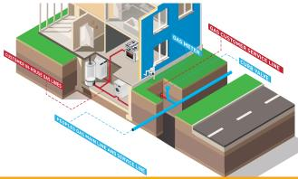
If your customer service line, house line, or gas appliance needs to be repaired or replaced, make sure the work is performed by a qualified installer. After the work is complete, following all rules and regulations, the installer must call Peoples so that we can test the line and complete our safety inspection. The qualified installer must also submit a "Service Installation Record (SIR)," available online as a mobile app. If the SIR is missing or incomplete, we cannot restore your gas service.
